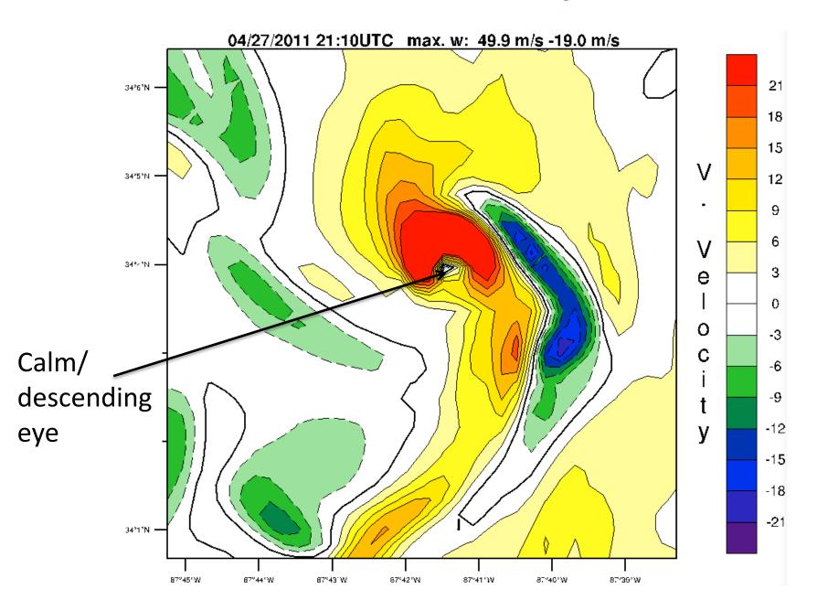
LES domain: Vertical velocity at 700m and 10m wind vectors
